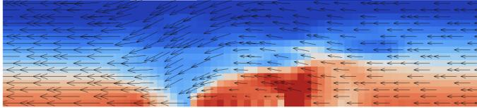
Figure 1: Pressure for a subduction model using Q1-P0 elements and averaged pressures. Notice that, even when averaging the pressures, there is an even-odd artifact centered on the bottom.
